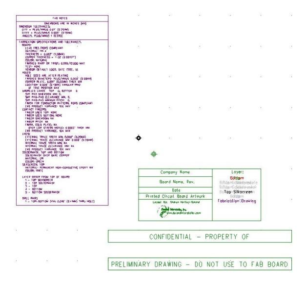
This particular set of Fab Notes deal with the most commonly used parameters of fabrication. Depending on your design, other elements may need to be specified. But, working from a basic list, you can easily add and delete elements as needed.
